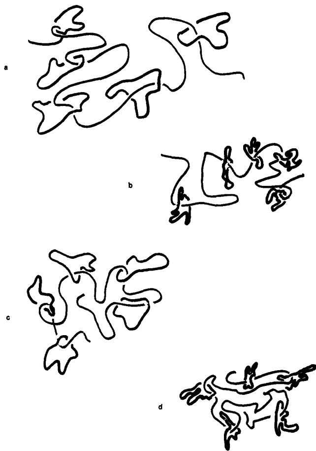
Figure 11. Solvent effects on polyrotaxane: (a) in a good solvent for both the cyclic and linear species, leading to expansion of both components; (b) in a good solvent for the linear macromolecule but a poor solvent for the cyclic species, leading to an expanded backbone but collapsed macrocycles; (c) in a poor solvent for the linear backbone but a good solvent for the macrocycle, providing a collapsed state of the linear component and an expanded state for the rings; (d) in a poor solvent for both the linear and cyclic components, affording collapsed conformations of both. The situation for b could lead to either smaller or larger total hydrodynamic volume than in c depending on the nature of the cyclic and linear species, the relative loading of the latter, and the solvent.
